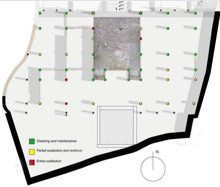
Figure 13. The appropriate disposal measures of the pillars in tea house's 1 floor
