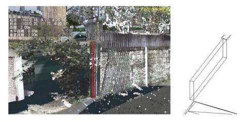
Figure 8 Neighbor building's fence height is reflected into the BIM model
